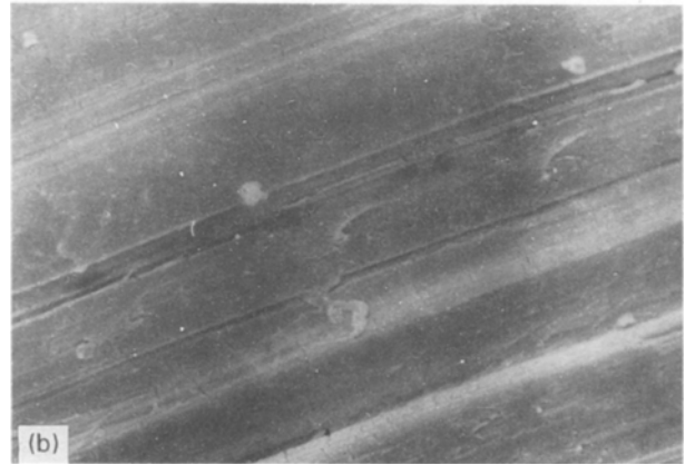
Figure 5 (a) Surface of the pull-out region of an untreated UHMW-PE fibre from the matrix, (b) surface of the pull-out region of a treated UHMW-PE fibre from the matrix.
